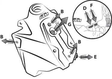
**Remove seat screw (B) and the screws on the side. Remove the tank screw (G), then empty any remaining fuel from the tank. Remove the (D/E/F) fasteners and remove the fuel pump.**
