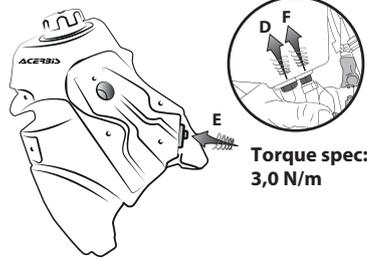
**On the fuel tank Acerbis (A), reconnect the fuel pump (E) with the original screws/hardware.**
