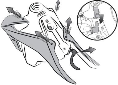
**Remove the radiator scoops. Disconnect the fuel pump cover cable and the fuel connector as indicated in the diagram. Inserire la vite nel foro della parte superiore del serbatoio.**
